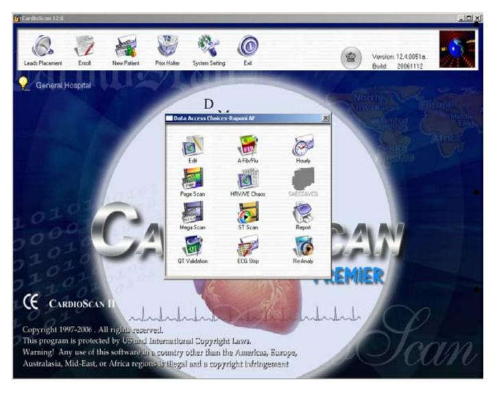
The A-Fib/Flu menu is mainly used to show you the detection of atrial fibrillation rhythm and the percent of time the patient is in A-Fib.
