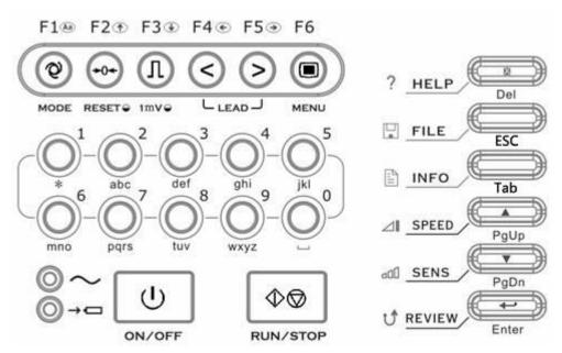
Figure 3-3 Control Panel of QRS-12
