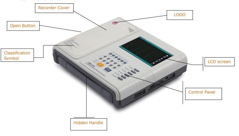
Figure 3-1 Front Panel of QRS-12
