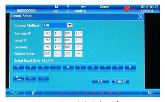
Figure 5-15 Communication Setting Interface
